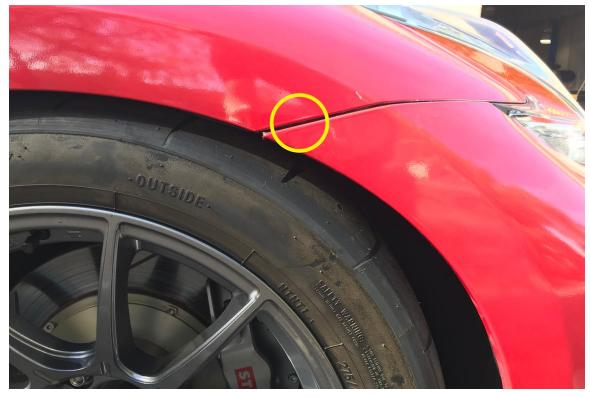
With the wheel turned in, you can push the fender liner out of the way slightly and gain access to the 10mm bolt.
