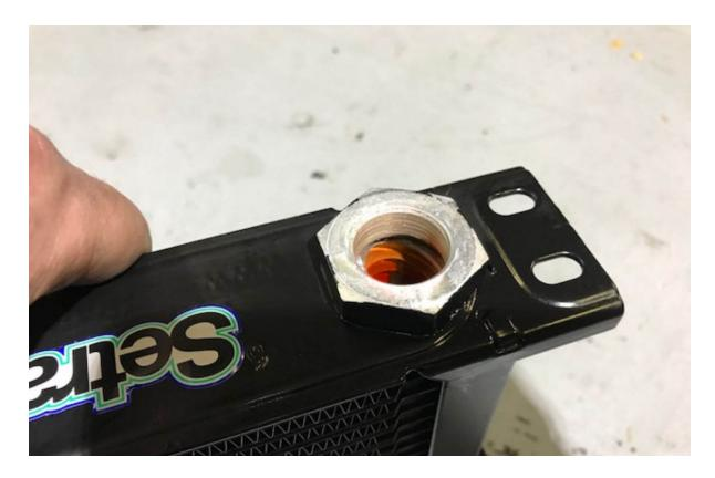
13. Apply a dab of fresh oil to the o-ring seal and thread the -6 AN to 22mm adapter fittings to the top of the cooler core and tighten them down. Take the 90 degree 3/8" push lock to -6AN fittings and thread them onto the top of the cooler loosely so they can be rotated later.
